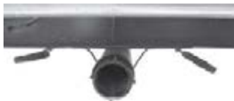
Black/Grey Tank Drain and Valves
