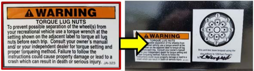
Lug nut torque pattern and warning label
